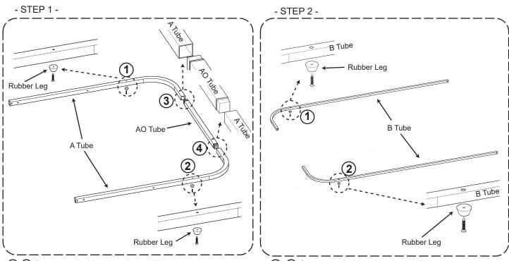
(1),(2) Screw up Rubber Leg into A Tube.
