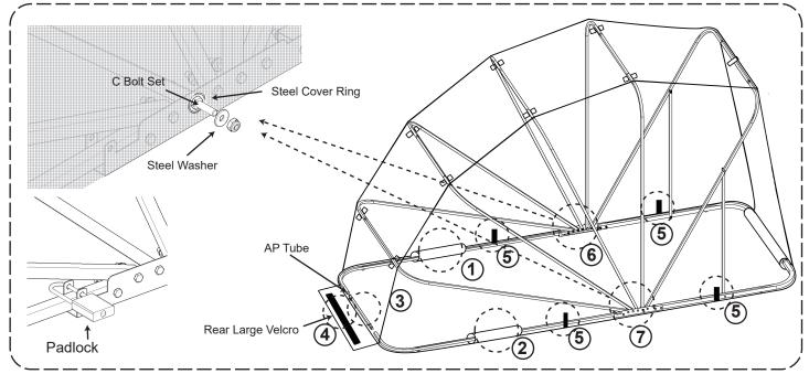
(1),(2) Put B Tube through pockets on left and right side of cover.
