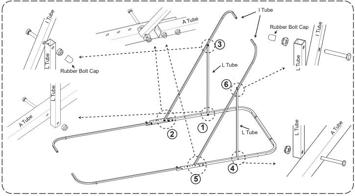
\* All bolts should be inserted from outside to inside of The Bike Shield.
