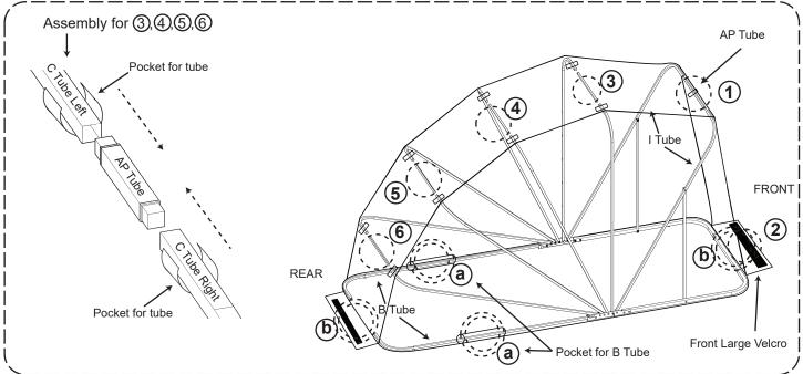
a) Identify front and rear side of the cover. Cover's rear side - Look up the position of two pockets for B Tube as shown.
