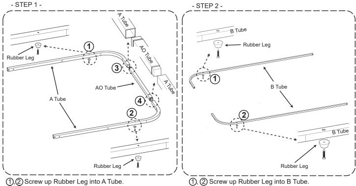
(3), (4) Connect AO Tube with two A Tube (right and left side).
